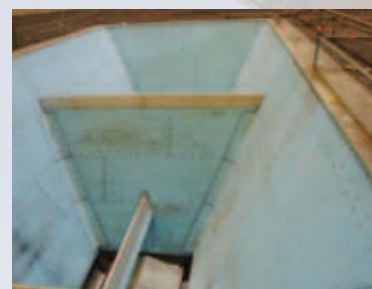
Fully Cladded Hoppers with TIVAR® BlueLine
