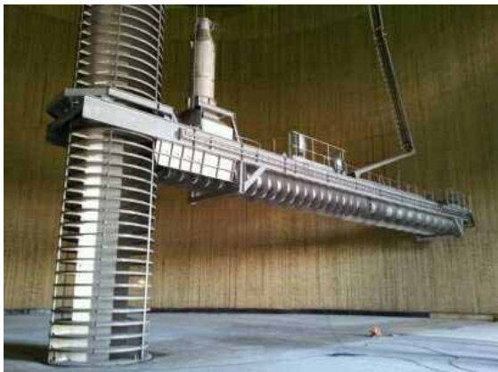
Eurosilos® system inside the Ammonium Sulfate silo
