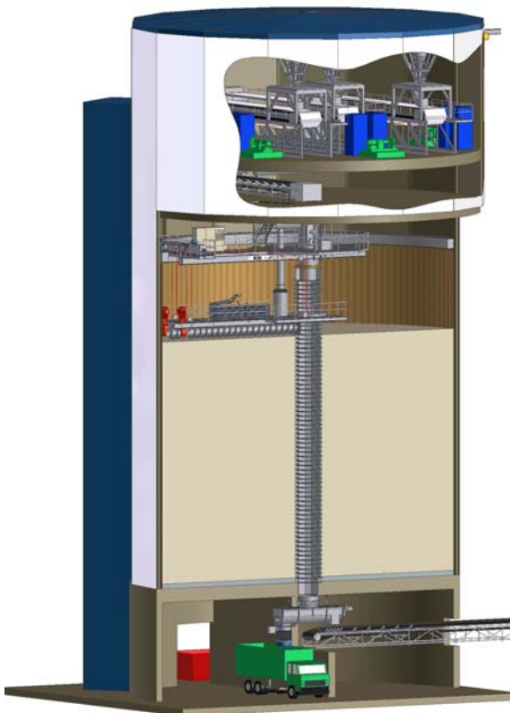
Fig. 1. Typical 10,000 m 3 FGD Gypsum Eurosilos ®
